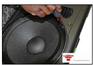
Step 11. – Use a pointed tool [such as an ice pick] to reopen holes for the grommets.
