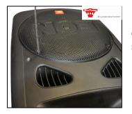
Step 1. – Place Cabinet on back and remove the four (4) Phillips screws fastening the grill.
